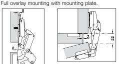
At opening angle of 90° and mounting plate height = 0 mm, the door swings out laterally 2 mm when opened.
